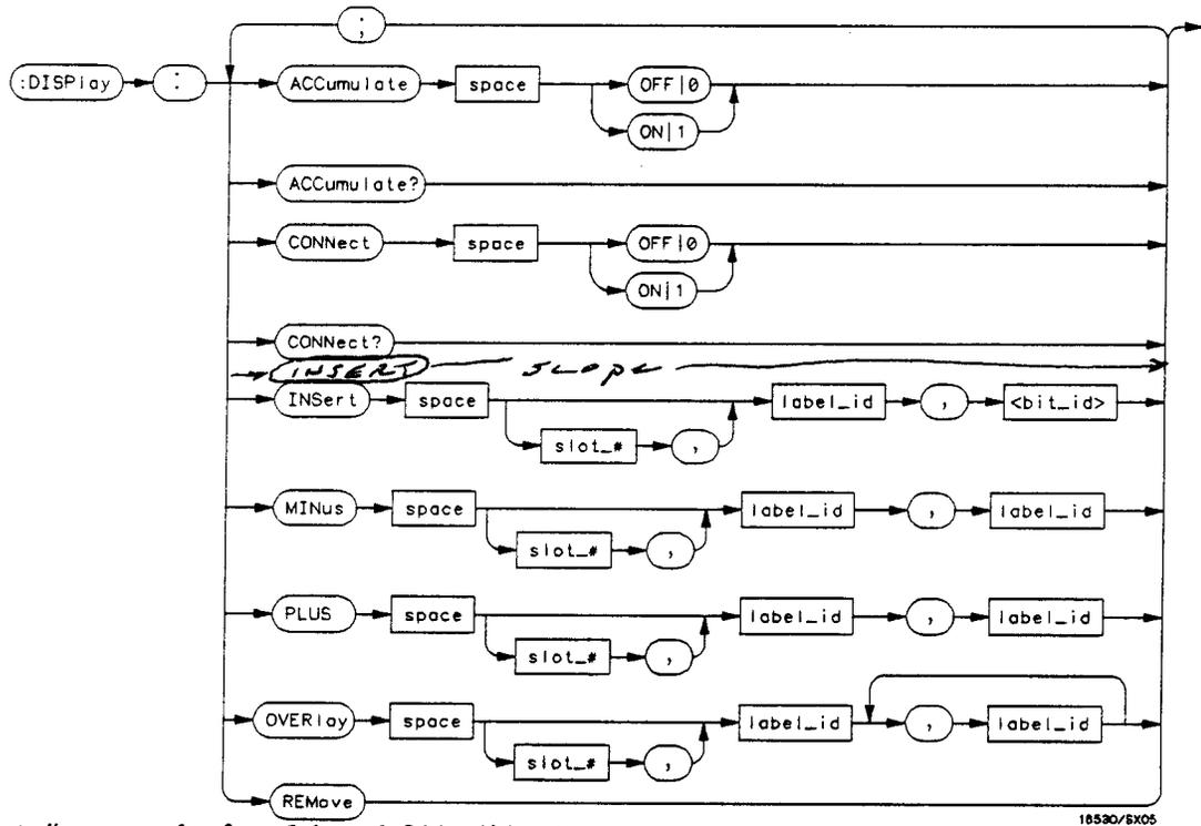
slot\_# = a number from 1 through 5 identifying the timebase card slot
