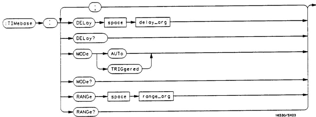
**delay\_arg** = delay time in seconds, from -2500 seconds through +2500 seconds
