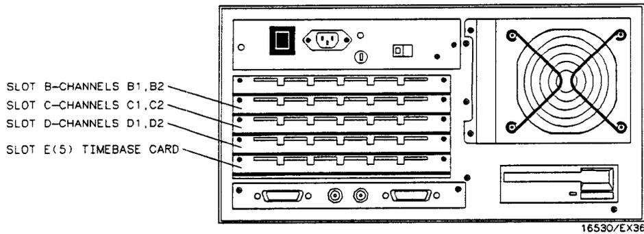
*Figure 5-2. Oscilloscope Label Identification.*
