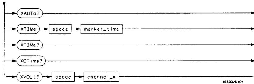
**channel\_#** = An integer from 1 through 8, depending on how many acquisition cards are installed.
