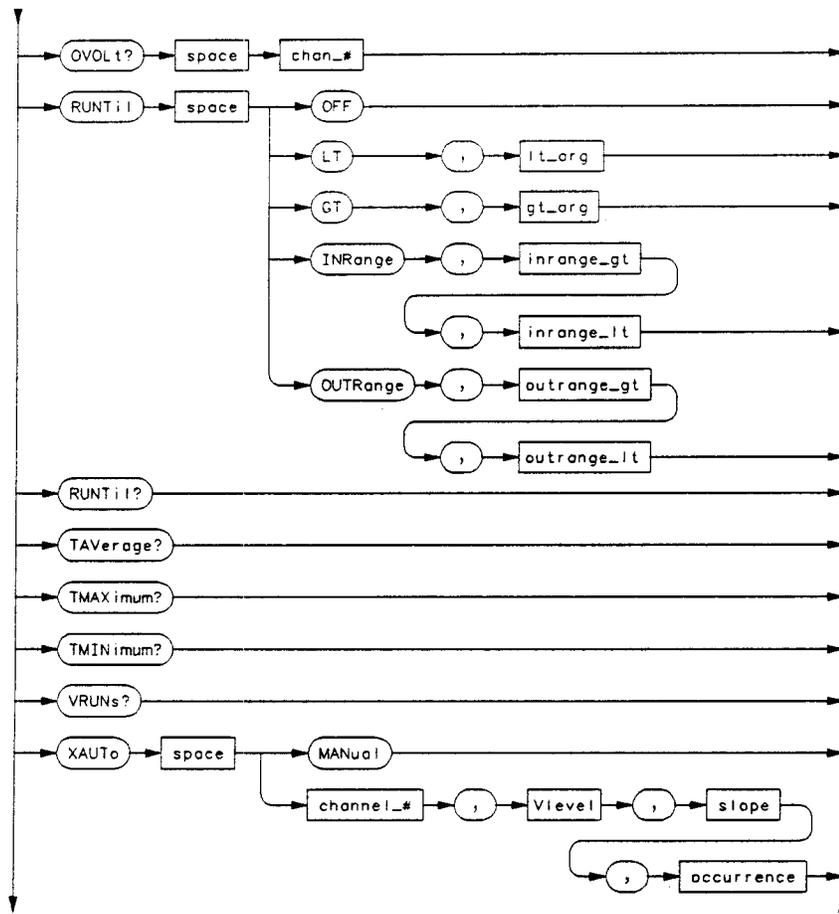
P/O Figure 6-1. MARKer Subsystem Syntax Diagram
